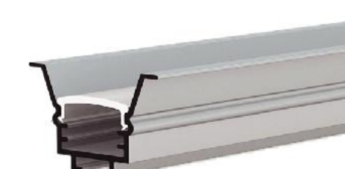
IC-177-AP2018 PC Ice white diffuser mask "A" Alu+Silky silver finish Thickness of PC: 0.85mm Thickness of Alu: 0.70mm
