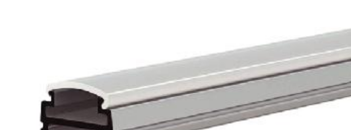
IC-077-AP1307 PC Ice white diffuser mask "A" Alu+Silky silver finish Thickness of PC: 0.80mm Thickness of Alu: 0.70mm
