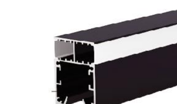
IC-151-AP2843 PC Ice white diffuser mask "A" Alu+Silky silver finish Thickness of PC: 0.80mm Thickness of Alu: 1.05mm
