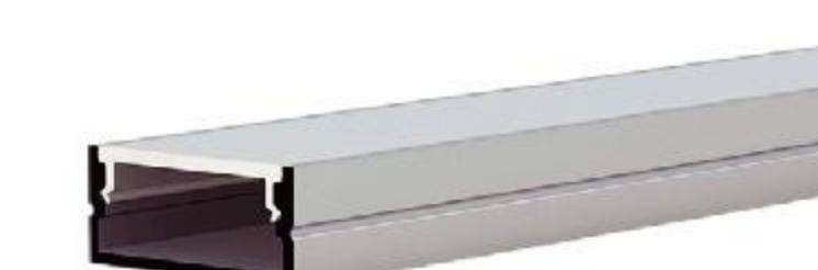
IC-012-AP2010 PC Ice white diffuser mask "A" Alu+Silky silver finish Thickness of PC: 0.85mm Thickness of Alu: 0.80mm
