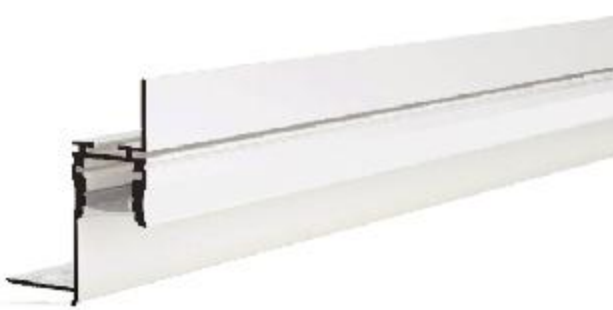
IC-318UP-PE5241 PC Ice white diffuser mask "A" Alu+Silky silver finish Thickness of PC: 0.90mm Thickness of Alu: 1.30mm
