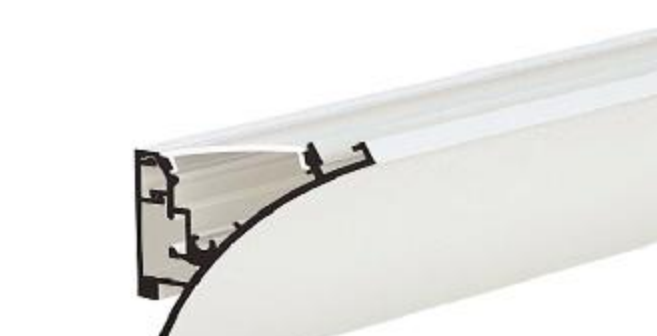
IC-354-AP5136 PC Ice white diffuser mask "A" Alu+Silky silver finish Thickness of PC: 0.90mm Thickness of Alu: 0.95mm
