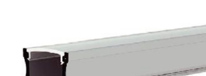
IC-061-AP1714 PC Ice white diffuser mask "A" Alu+Silky silver finish Thickness of PC: 0.85mm Thickness of Alu: 0.85mm
