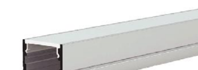
IC-065-AP2015 PC Ice white diffuser mask "A" Alu+Silky silver finish Thickness of PC: 0.85mm Thickness of Alu: 0.75mm
