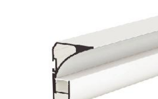
IC-047-AP6037 PC Ice white diffuser mask "A" Alu+Silky silver finish Thickness of PC: 0.80mm Thickness of Alu: 1.30mm
