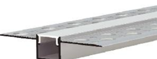
IC-330UP-PE1313 PC Ice white diffuser mask "A" Alu+Silky silver finish Thickness of PC: 0.75mm Thickness of Alu: 0.95mm
