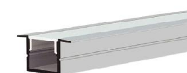
IC-083W-AP1010 PC Ice white diffuser mask "A" Alu+Silky silver finish Thickness of PC: 0.80mm Thickness of Alu: 0.70mm
