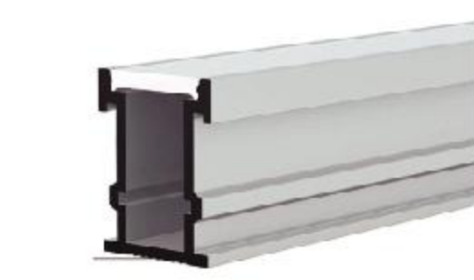
IC-231-UL2126 PC Ice white diffuser mask "A" Alu+Silky silver finish Thickness of PC: 2.60mm Thickness of Alu: 1.25mm
