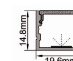
IC-065-AP2015 PC Ice white diffuser mask "A" Alu+Silky silver finish Thickness of PC: 0.85mm Thickness of Alu: 0.75mm
