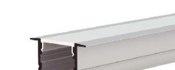
IC-065W-AP2015 PC Ice white diffuser mask "A" Alu+Silky silver finish Thickness of PC: 0.85mm Thickness of Alu: 0.75mm
