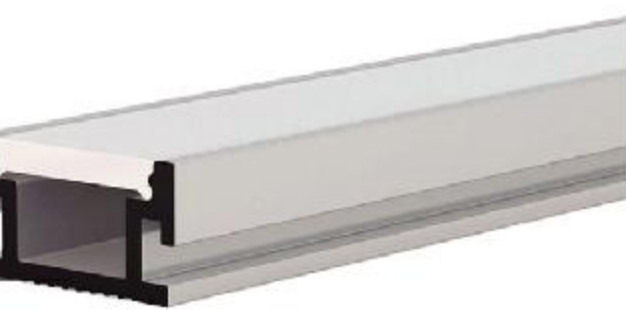
IC-212-UL2111 PC Ice white diffuser mask "A" Alu+Silky silver finish Thickness of PC: 2.60mm Thickness of Alu: 1.15mm
