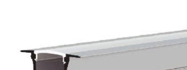
IC-061W-AP1714 PC Ice white diffuser mask "A" Alu+Silky silver finish Thickness of PC: 0.85mm Thickness of Alu: 0.85mm
