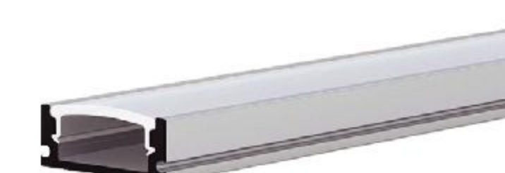
IC-070-AP1707 PC Ice white diffuser mask "A" Alu+Silky silver finish Thickness of PC: 0.85mm Thickness of Alu: 0.70mm
